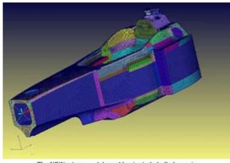
The NEINastran model used laminated shell elements and solid elements for foam-filled areas.
