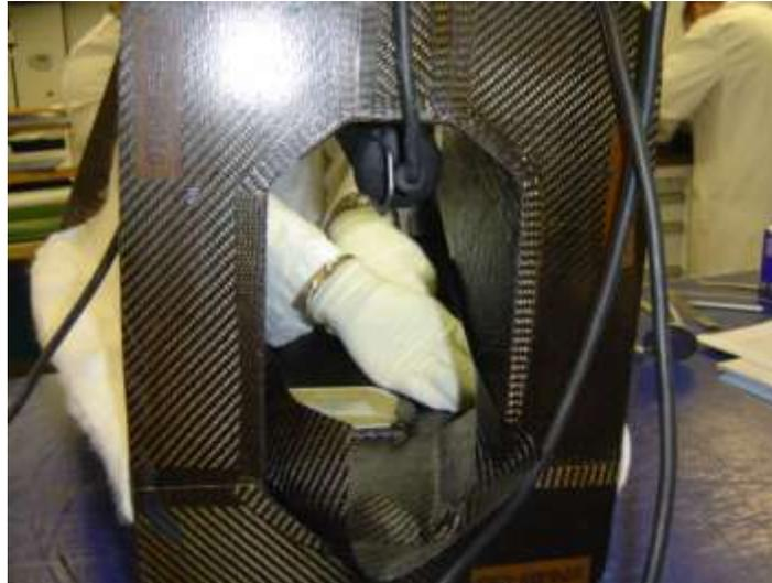
Figure 24: Hand laminating with pre-preg.
