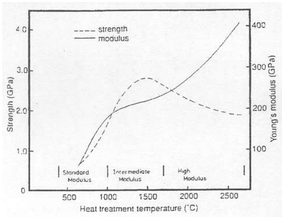
Figure 19: Relationship between heat treatment temperature and mechanical properties of PAN-based carbon fibres.
