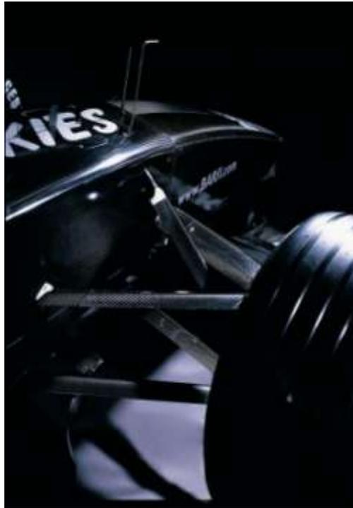
Figure 17: Composite suspension.
