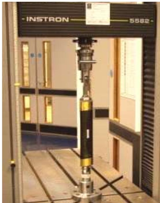
Figure 9: Rear push rod – compression member.
