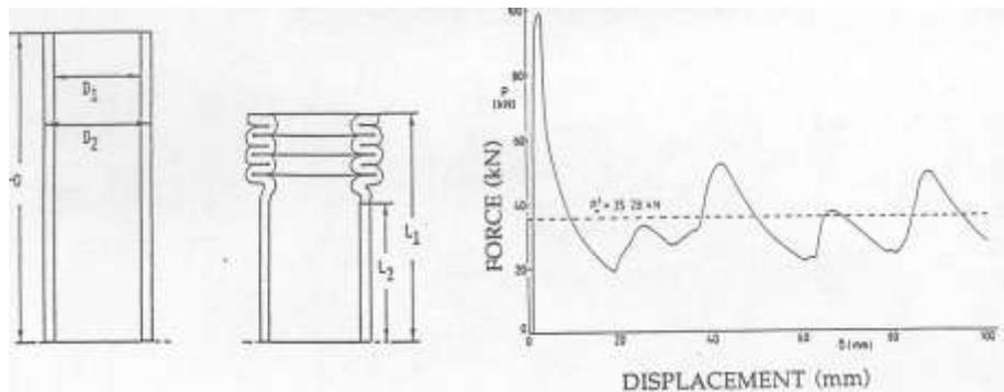
Figure 34: Energy absorption by metallic structures.
