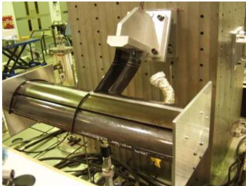
Figure 10: Rear wing, loaded in bending.
