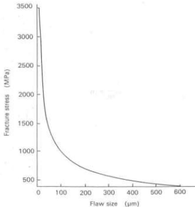
Figure 7: Relationship between flaw size and failure stress of a material (2).
