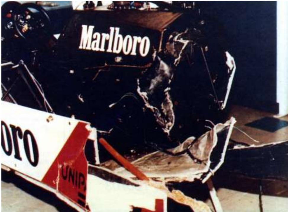
Figure 15: MP4/1 chassis following large impact.
