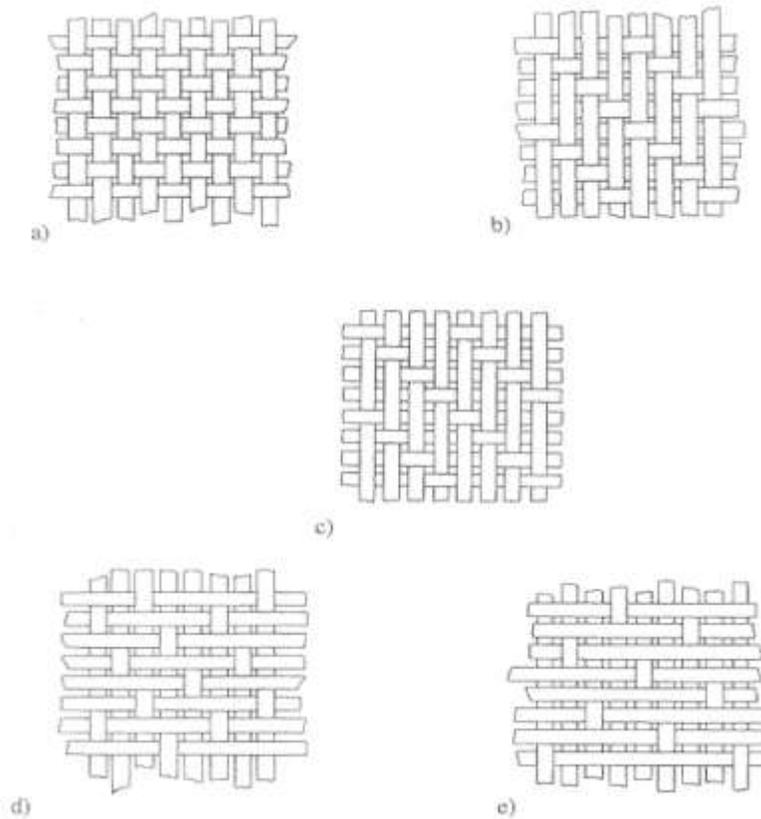
**Figure 21:** Fabric styles commonly used in composites:
