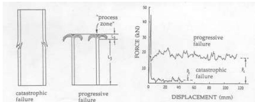
Figure 35: Energy absorption by composite structures.
