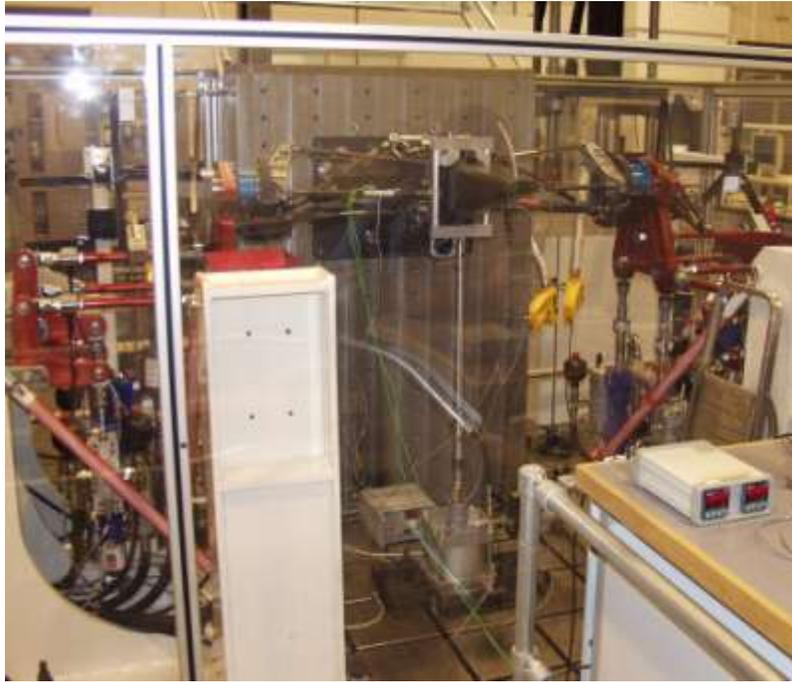
**Figure 23:** Strength, stiffness and durability testing on a composite gearbox and rear suspension assembly.
