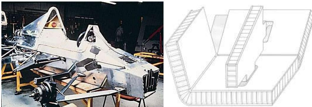
Figure 13: "Cut and fold" aluminium honeycomb chassis (late 1970's).
