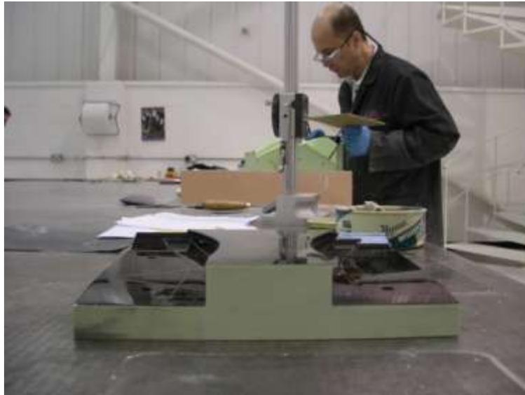
Figure 29: Finished patterns prepared for moulding.
