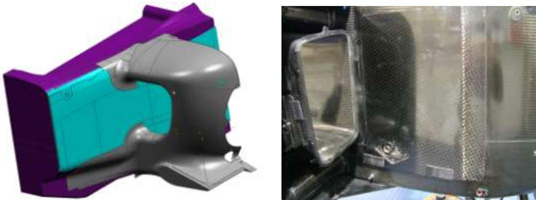
Figure 20: Zylon appliqué armour panel.
