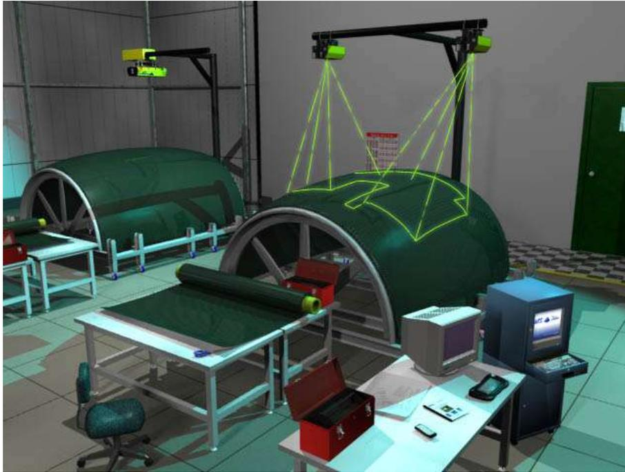
Figure 27: Laser projections to aid ply placement.
