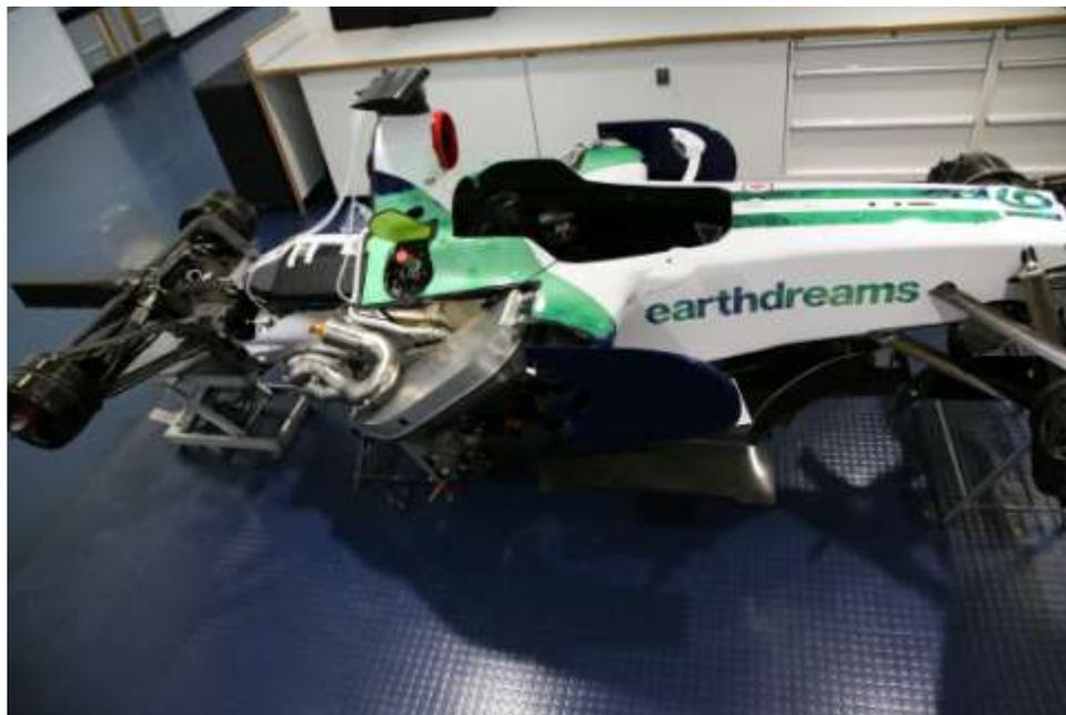
Figure 3: The "primary structure" of a formula 1 car consists of chassis, engine and gearbox.
