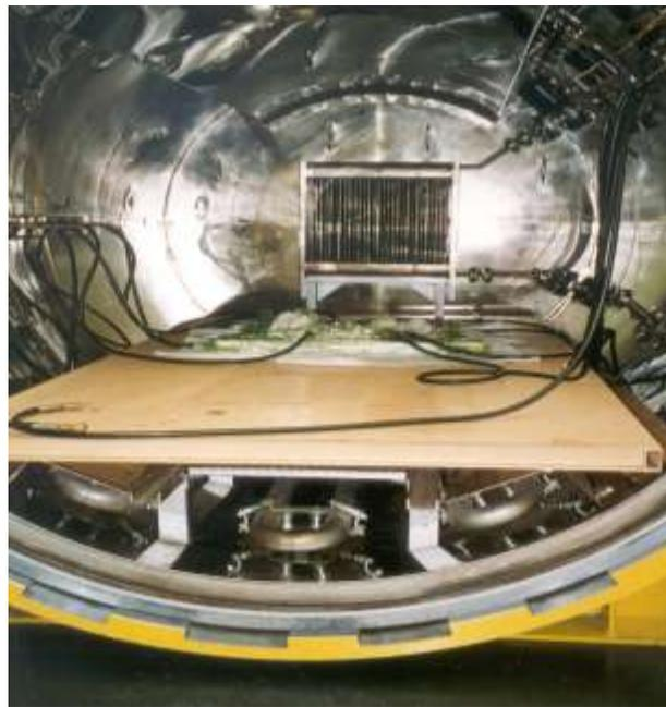
**Figure 32:** Autoclave cure.
