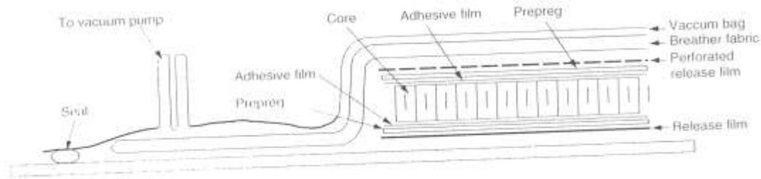
**Figure 31:** Composite curing assembly.
