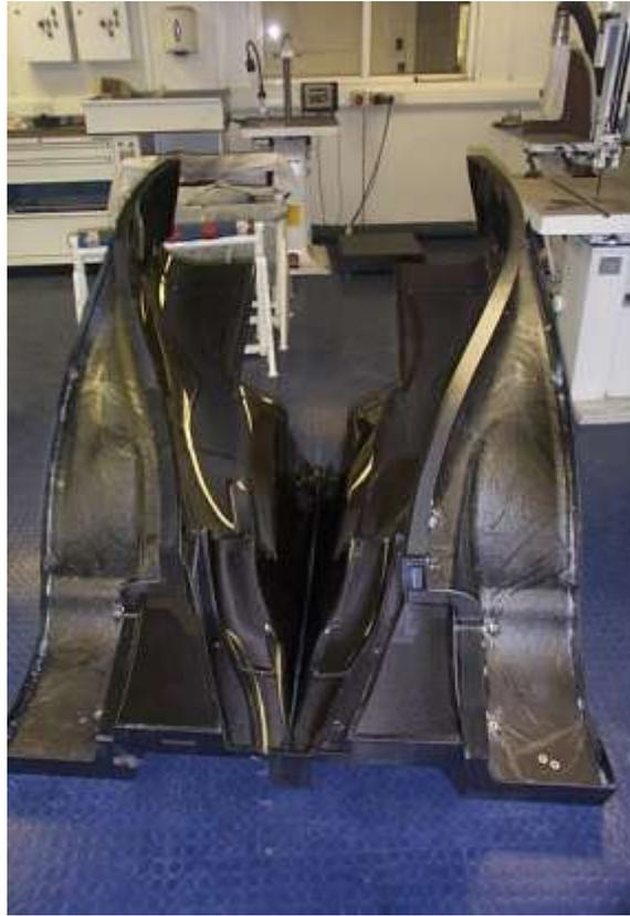
Figure 30: Composite engine cover mould.
