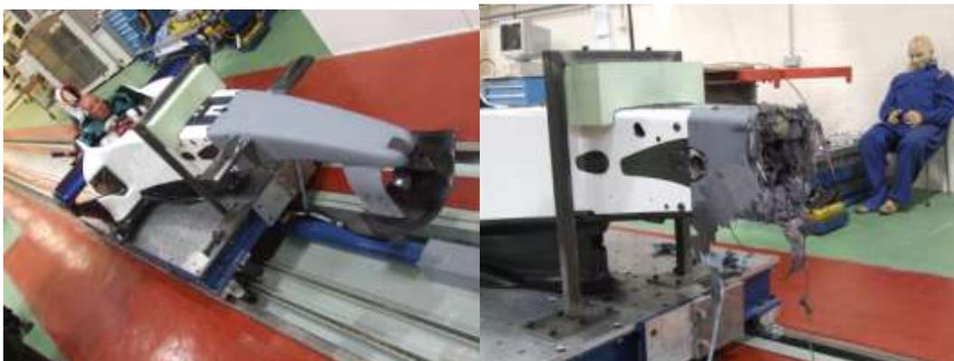
Figure 36: FIA nose crash test.
