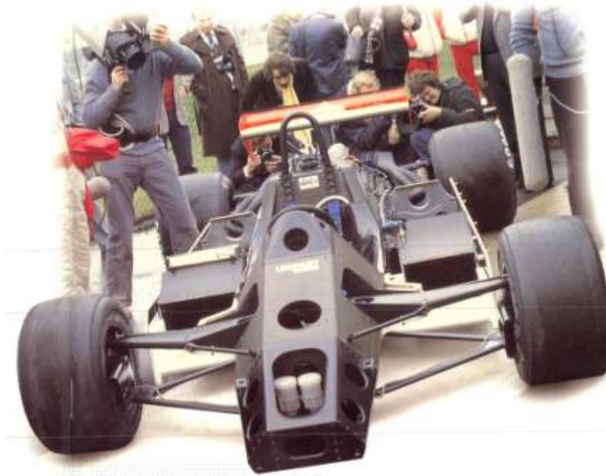
Figure 14: The first carbon monocoque McLaren MP4/1 (1980).
