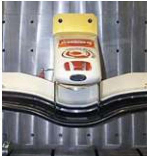
**Figure 8:** Front wing pillars, loaded in tension.
