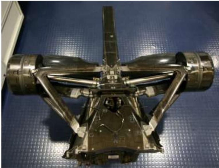
Figure 2: Gearbox and rear suspension.
