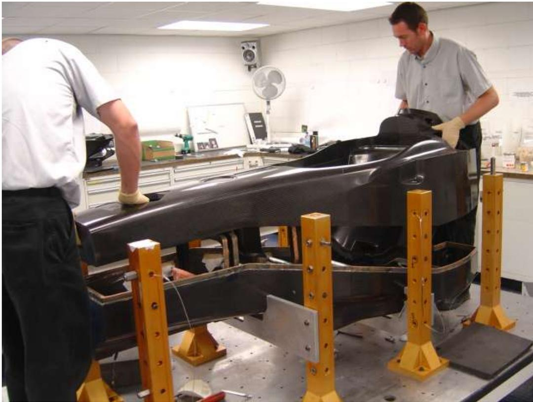
Figure 33: Chassis assembly.
